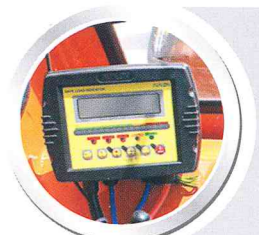
SLI Monitoring System
